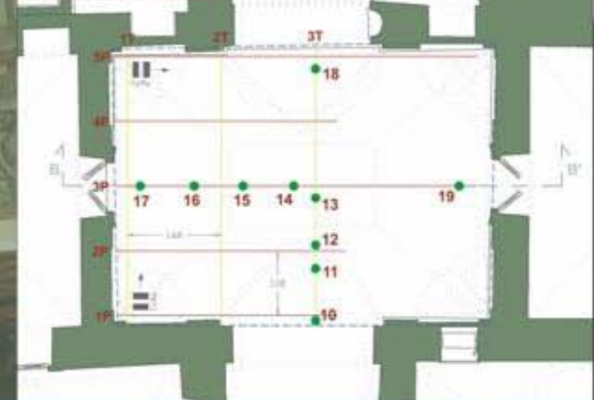
PLAN WITH GPR PROFILES
