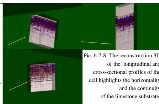
Pic. 6-7-8: The reconstruction 3D of the longitudinal and cross-sectional profiles of the cell highlights the horizontality and the continuity of the limestone substrate.
