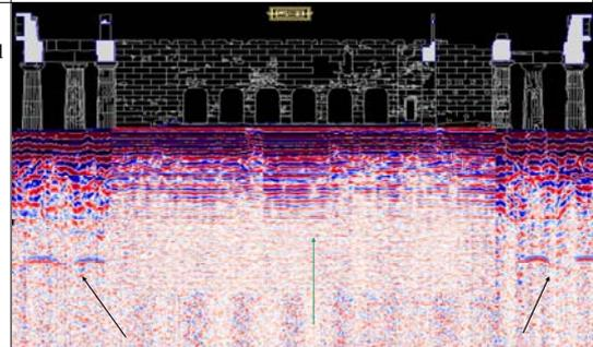
Pic. 5: Section of the foundations, along the greater axis of the temple: the black arrows indicate the kerbs, while the green arrow the horizontal natural substrate.
