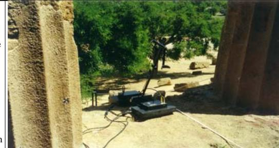
Pic. 2: PulsEkko 1000: instrument used for the geophysical survey.
